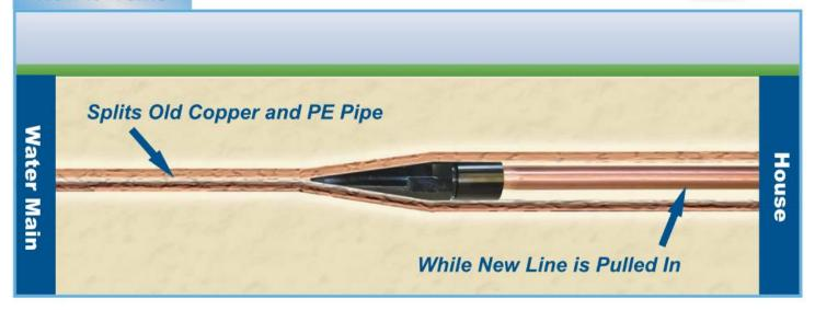
The Wedge service line replacement tool is ideal for replacing 3/4" and 1" water services quickly and easily. Operation of the Wedge is simple - just feed the aircraft cable through the existing service and then pull the Wedge through the ground using a backhoe, truck or winch. No special equipment is required! The new service can be easily attached to the back of the Wedge so the old line can be split or pulled out and the new line pulled in, all in one operation!
