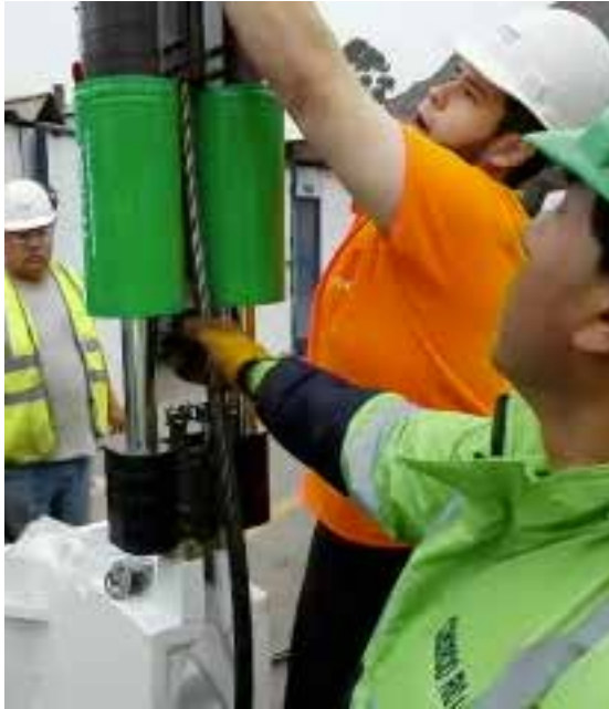
Figure 5 Inserting cable to upper grippers
