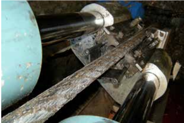
Figure 14 Cable out of alignment with retaining (lower) grippers
