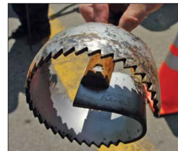
Stege Sanitary District uses a SRECO-Flexible root cutter to clean sewer lines in El Cerrito, Calif.
