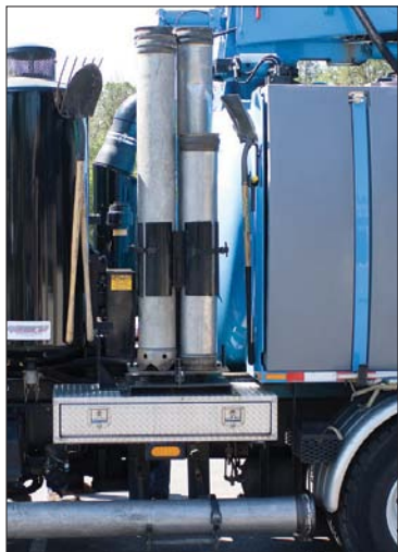
General Equipment Company built a lazy Susan holder for sections of vacuum tube on Clean Water Services’ Aquatech combination trucks.
