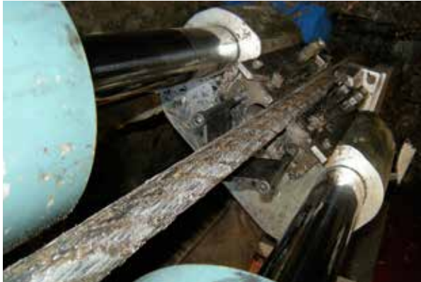
Figure 13 Cable out of alignment with retaining (lower) grippers
