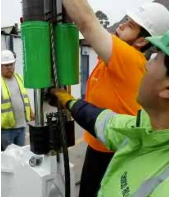
Figure 4 Inserting cable to upper grippers
